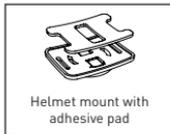
Use the helmet mount with the double-sided adhesive pad to attach it to helmets without air vents. Stick the double-sided adhesive pad to the bottom of the helmet mount. When attaching the mount, be sure the adhesive pad is stuck to a smooth surface. The surface needs to be clean and free of any grease. Be sure it is securely in place before every activity.
