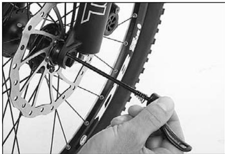
5. Place the springs and the nuts on the bolt. Turn the right end now protruding from the hub and the nut clockwise.
