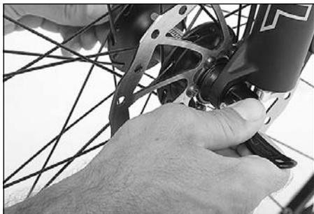
8. Now turn the nut or the Allen key bolt head until the eccentric lever, when turned around its bearing more than 90° to meet slight resistance (it now forms an approximately straight line extension of the hub axis).
