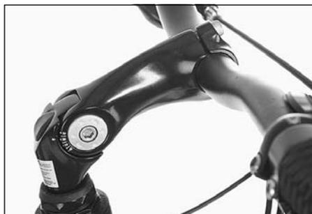
Many bikes are fitted with an adjustable stem, the height and angle of which can be adjusted. Only have adjustment carried out in a specialist workshop!
