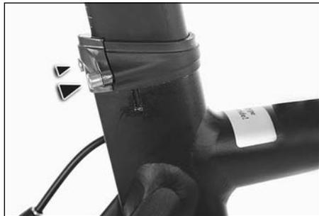
For clamping without a quick release a hexagon socket and a torque wrench of the appropriate size are required. Please also consult your dealer.
