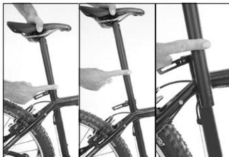
6. Turn the saddle so that the saddle points in the direction of travel.
