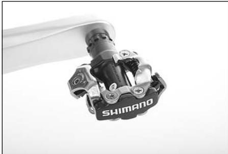
With click-in pedals the shoe and pedal are firmly connected in a vertical direction. When pedalling you can not only push the pedal down but also pull it upwards. To be able to use a click-in pedal to the full you need shoes specially designed for the pedal system concerned and to which the pedal hooks supplied with the pedal can be affixed.
