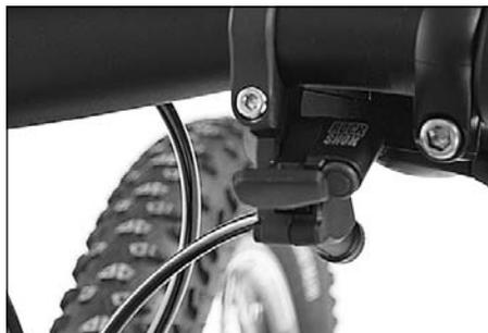
2. If your forks have a fixed adjustment mechanism as shown in the illustration, please read its instructions in the suspension fork manufacturer's component instructions.
