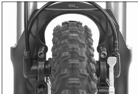
1. Check correct fixing and screw connections of the entire brake system:
