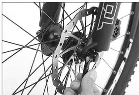
2. Turn the nut counter-clockwise until the wheel can be removed from the frame or front forks without any great effort. Should the nut come right off the screw please ensure that the little springs do not get lost.
