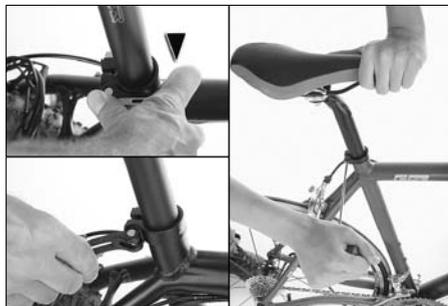
2. Withdraw the saddle with seat post from the frame.
