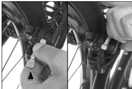
10. Please ensure that the brake blocks correctly cover the rim shoulder when operated.
