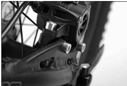
*Incorrect tightening* A loose screw can often be recognised by a projecting screw head.
