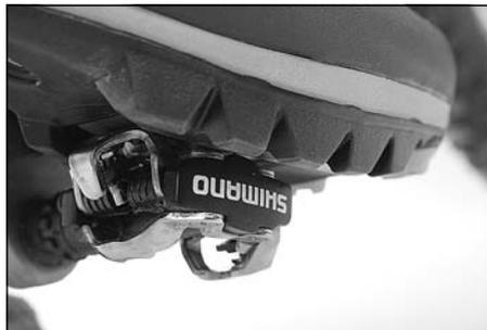
The shoe is now firmly vertically connected with the pedal. Depending on the pedal system the shoe has sideways freedom of movement.
