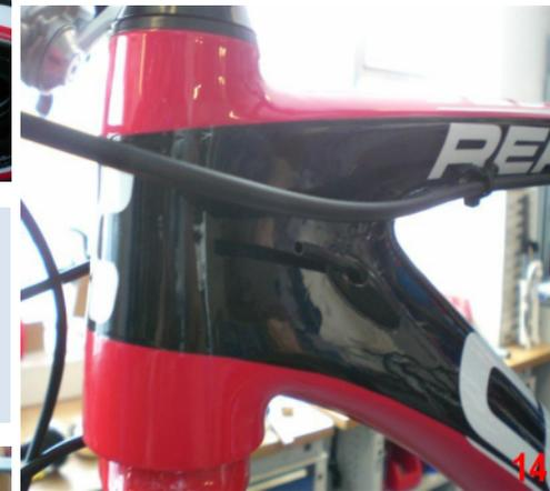
Finally you pin the cable of the front derailleur through the little hole of the bottom bracket housing. After that you put on the sealing and fix the cable with the screw of the front derailleur correctly.
