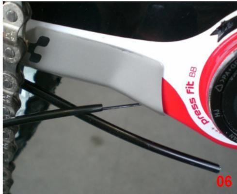
After that please do not drag the shifting cable completely out, otherwise you will get in trouble to mount a new cable into the frame. By slotting the old shifting cable into a liner (about 1m long) and carry the liner through the right hole on top of the downtube, you can remove the old cable. **If this shouldn't be possible instantly, you can simplify the working step by disassembling the fork.** (6-7)
