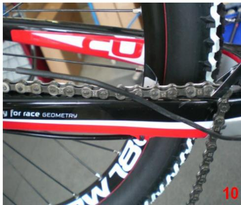
Now you thread the liner (20cm) on the new shifting cable, slide on the cable stroke and insert it into the chainstay. Finally you have to slide on the cable housing and screw the shifting cable to the rear derailleur. (10-11)
