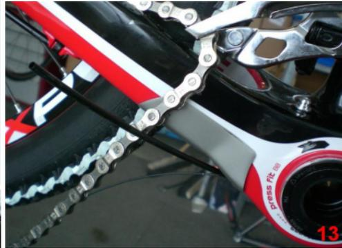
Further you pull the liner out of the upper downtube, like it's described on page 5 to 6. By disassembling the fork the procedure will be simplified a lot.
