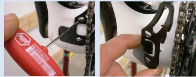
«« first loosen the 2.5mm allen wrench screws of the anti-chainsuck-cap and remove the cap
