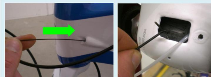
«« Now you put the cable through the down tube until you can pull it out of the hole at the BB shell.
