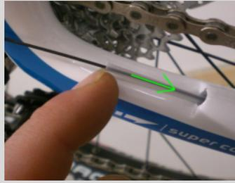
«« Pull the cable out of the cable exit.
