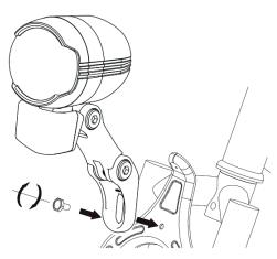
Attach the headlamp ① to the bicycle using a bracket ⑤ and ensure that the headlamp cannot shift on its own again [5Nm].
