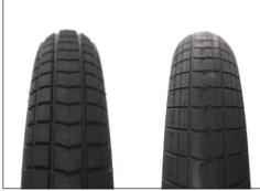
**Bild:** Optimum tyre tread (left); Worn tyre tread (right)
